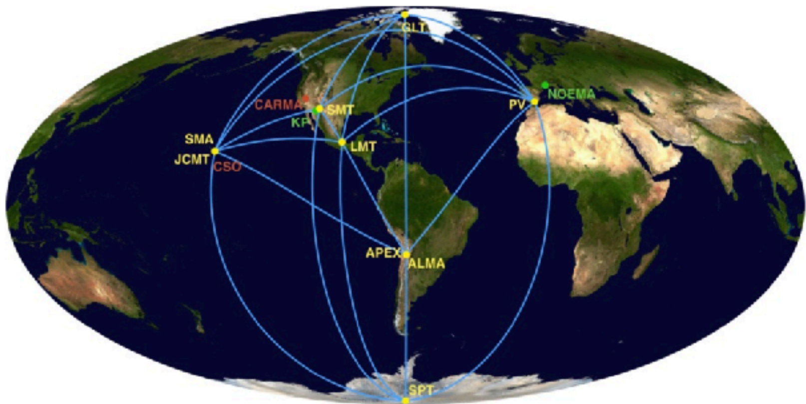
Figure 2. A map of the EHT. Stations active in 2017 and 2018 are shown with connecting lines and labeled in yellow, sites in commission are labeled in green, and legacy sites are labeled in red. From Paper II (Figure 1).
