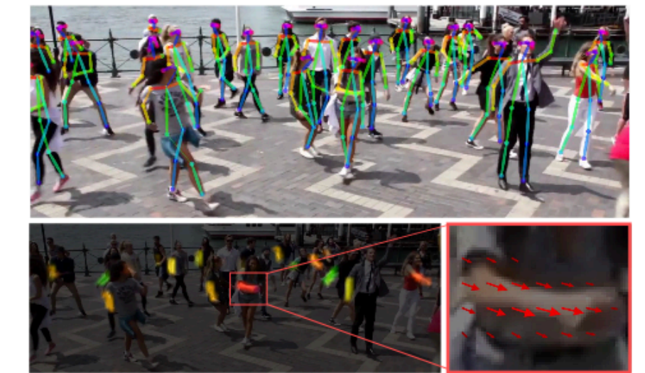
Figure 1. Top: Multi-person pose estimation. Body parts belonging to the same person are linked. Bottom left: Part Affinity Fields (PAFs) corresponding to the limb connecting right elbow and right wrist. The color encodes orientation. Bottom right: A zoomed in view of the predicted PAFs. At each pixel in the field, a 2D vector encodes the position and orientation of the limbs.
